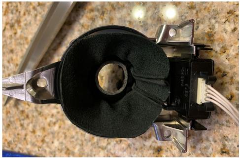
viii. After some time, remove the shift knob. Unfasten the EDC trim and separate the leather boot from the EDC trim piece and gear selector. You will see a compressed ring mark on the leather where it was clamped in place.
