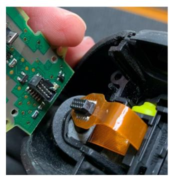
iii. Many gear selectors look identical, but the internals vary. The correct gear selector has the little door located as shown in the image below. The E70 gear selector has the same door feature. There is a ribbon cable that goes from the circuit board in the shift knob to a circuit board located behind that plastic door. If the F-Series gear selector has this door, then it is very likely that it also has a similar ribbon cable and connector as the E70.
