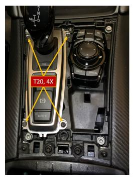
vii. The assembly that is left is actually made of two pieces, one is the gear selector and the other is a frame. Remove the three (3) T25 screws to separate the frame from the gear selector. One
