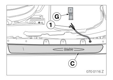
All cars (illuminated version only) Connect plug contacts (1) of door sill strip **C** into plug casing **G**, pin 1 and pin 3 (cables for pin 1 and pin 3 can be selected as required).
