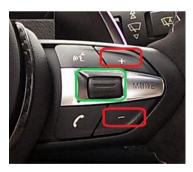
It can be done by pressing and holding **volume** + and **volume** – keys for 6-7 seconds. Backlight on the steering wheel will blink when mode is changed. Configuration will be retained after switching ignition off.
