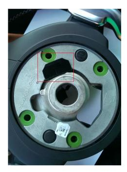
2. Drill a hole (red mark on picture below) and screw a bolt
