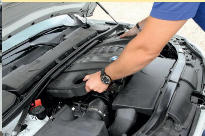
The large cover conceals an insulation mat that also has to be removed carefully.
