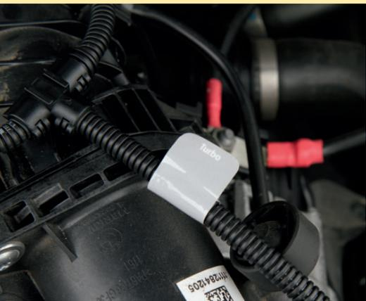
The individual lines of the Diesel Power system have even been labelled to prevent wrong connections!
