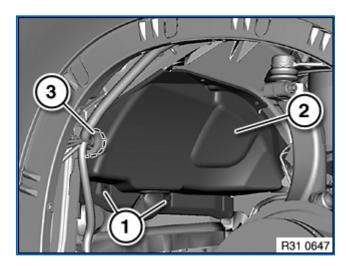
Installation note: When installing, make wiring harness penetration (3) is in correct position.
