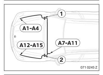
Route branches **A1–A4** and **A7–A15** as follows along the standard wiring harness:
