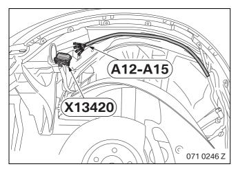
Route branches **A12–A15** along the standard wiring harness to plug **X13420** of the left headlight.
