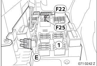
Insert blade terminal fuses **E** into slots F22 and F25 of the front fuse holder (1).
