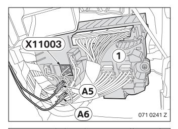
Connect branches **A5–A6** as follows to plug **X11003** (SW 6-pin) on the front fuse holder:
