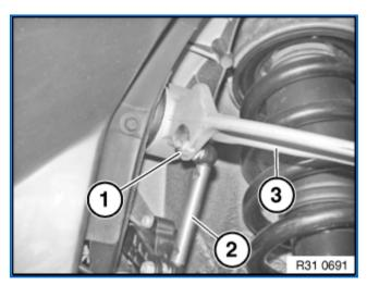
Slacken nut (1). Remove jointed rod (2) from upper wishbone (3).
