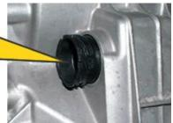
4. Pull the sealing sleeve locking mechanism to the unlocked position and remove the sealing sleeve.
