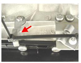
Use a wire tie or mechanics wire and secure the emergency release lever in a slight backwards position as shown.
