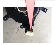
12 pin connector plugged into New coil spring. Old coil spring Has a 6 pin.
