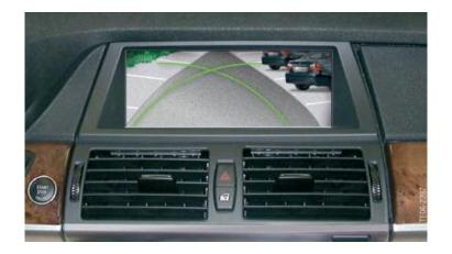
Only the relevant turning circle line is shown as soon as the driver turns the steering wheel. The opposite turning circle line is blanked out depending on the steering lock and is no longer shown at full lock.
