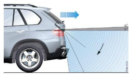
Increasingly only the upper area of the image (from about 1m distance from the vehicle up to a minimum angle of 10° above the horizontal) is shown on the screen when rear-view at faster speed (more than 3 mph)
