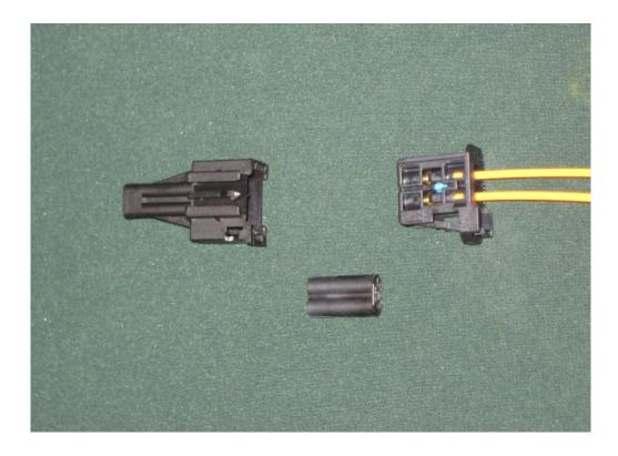
Now simply terminate your unused MOST connector by plugging it in to the MOST terminator
