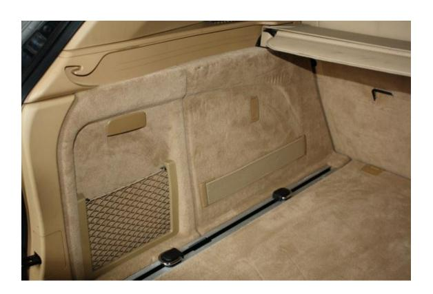
Remove the left side cover as shown on the pictures. Please note that there will be 4 plastic clips around the cover which needs to be removed.
