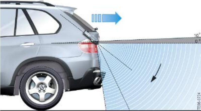
Increasingly only the upper area of the image (from about 1m distance from the vehicle up to a minimum angle of 10° above the horizontal) is shown on the screen when rear-view at faster speed (more than 3 mph)
