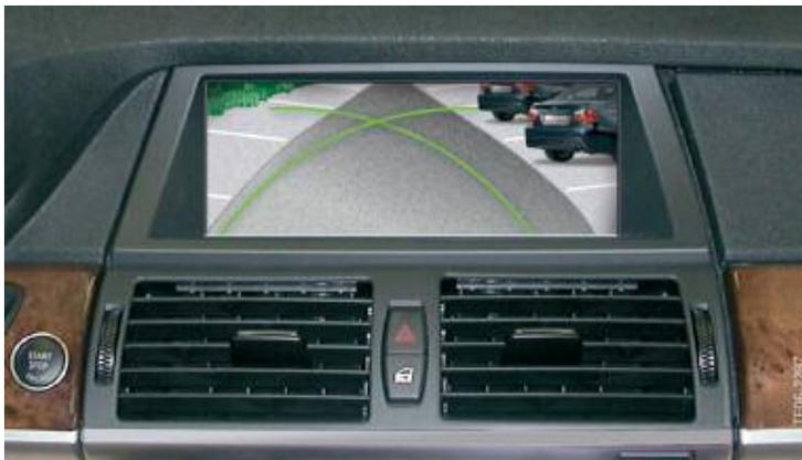
Only the relevant turning circle line is shown as soon as the driver turns the steering wheel. The opposite turning circle line is blanked out depending on the steering lock and is no longer shown at full lock.
