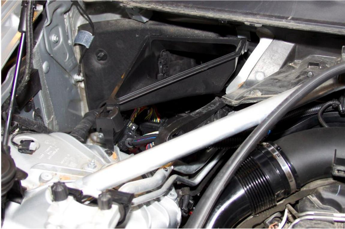
Control Module Install 14 - Ziptie the control module to the nearby wiring
