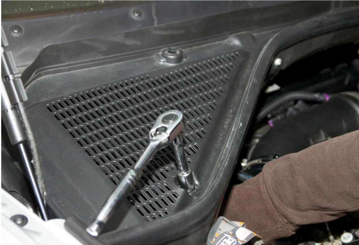
**Control Module Install 1 - The HVAC area will keep the control module nice and dry. We need to loosen the HVAC cover to install the control module. These black nuts require a 13mm socket, and you can only get a quarter turn out of them.**
