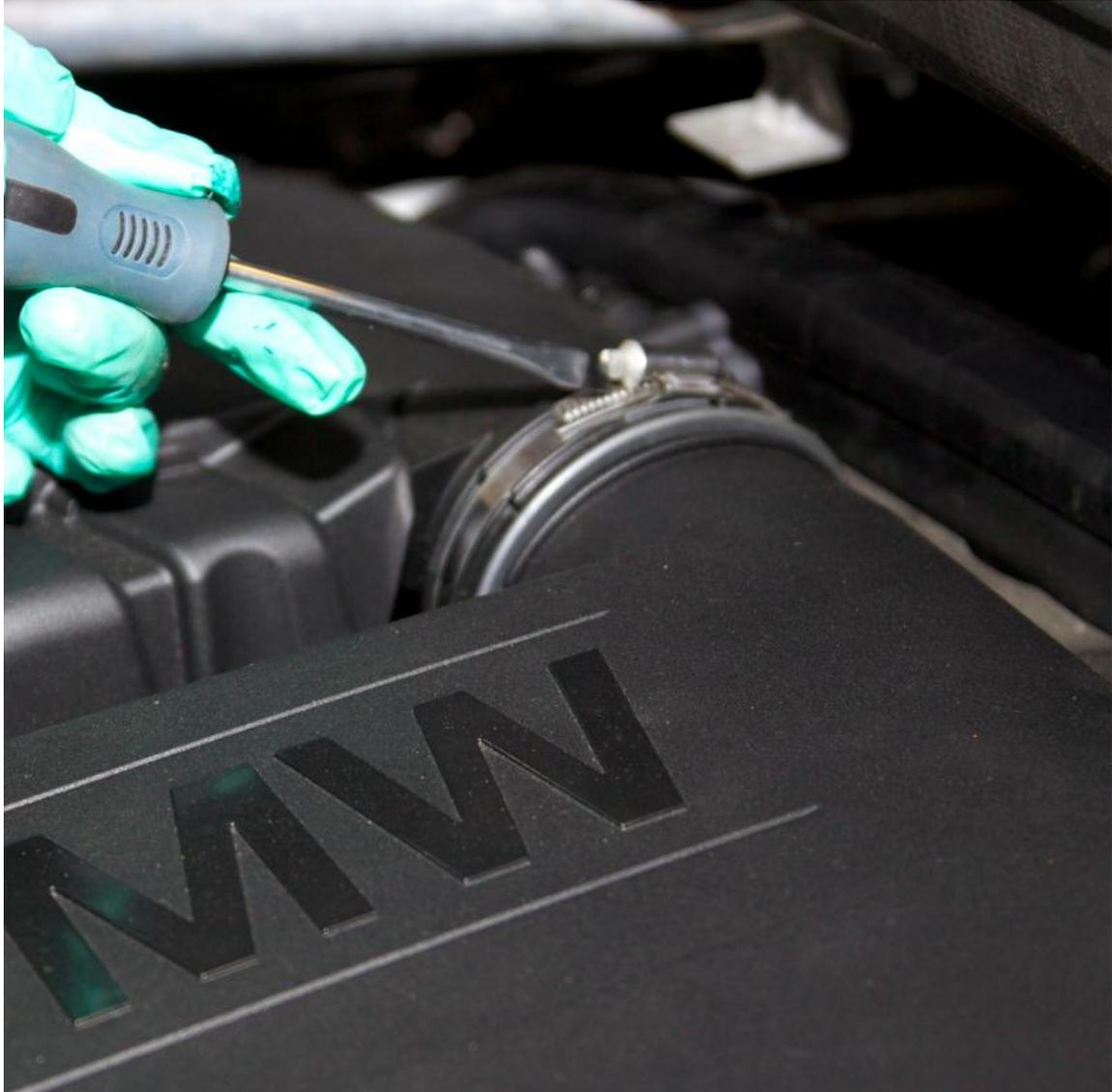
Air Box 1 - Loosen the clamp
