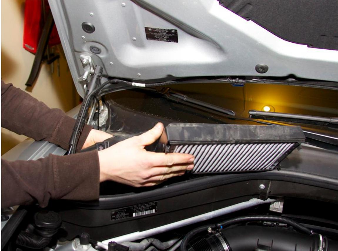
**Control Module Install 4 - Make sure you unplug the cabin air filter plug before taking out the cabin air filter housing**
