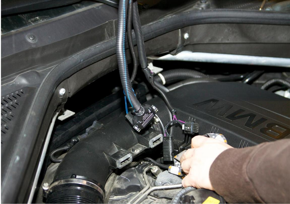
Sensor Three 2 Harness Routing Example
