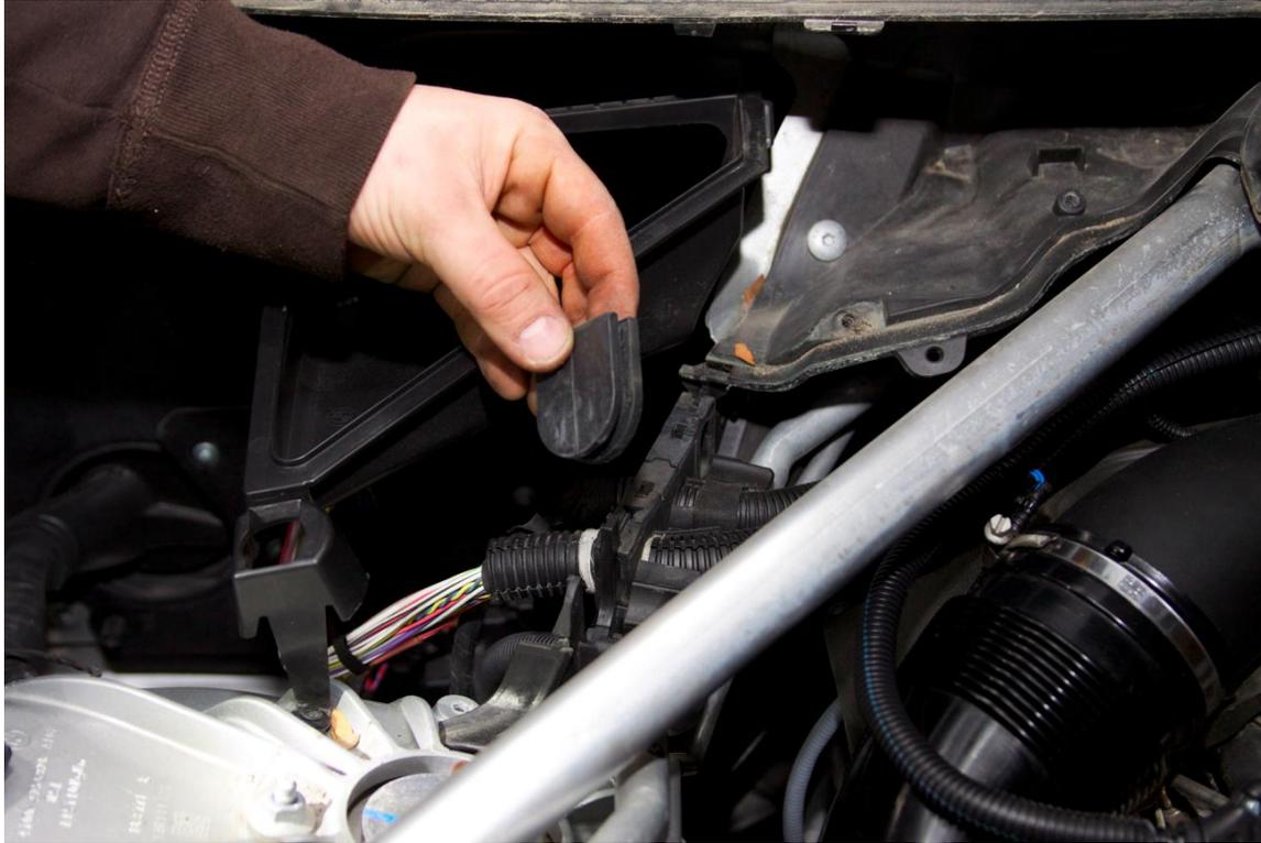
**Control Module Install 10 - There is an unused rubber plug. Take it out.**
