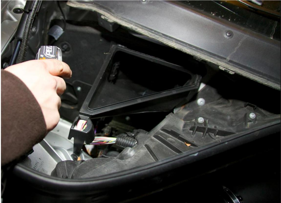
Control Module Install 5 - Take off the weather strip and the engine compartment divider
