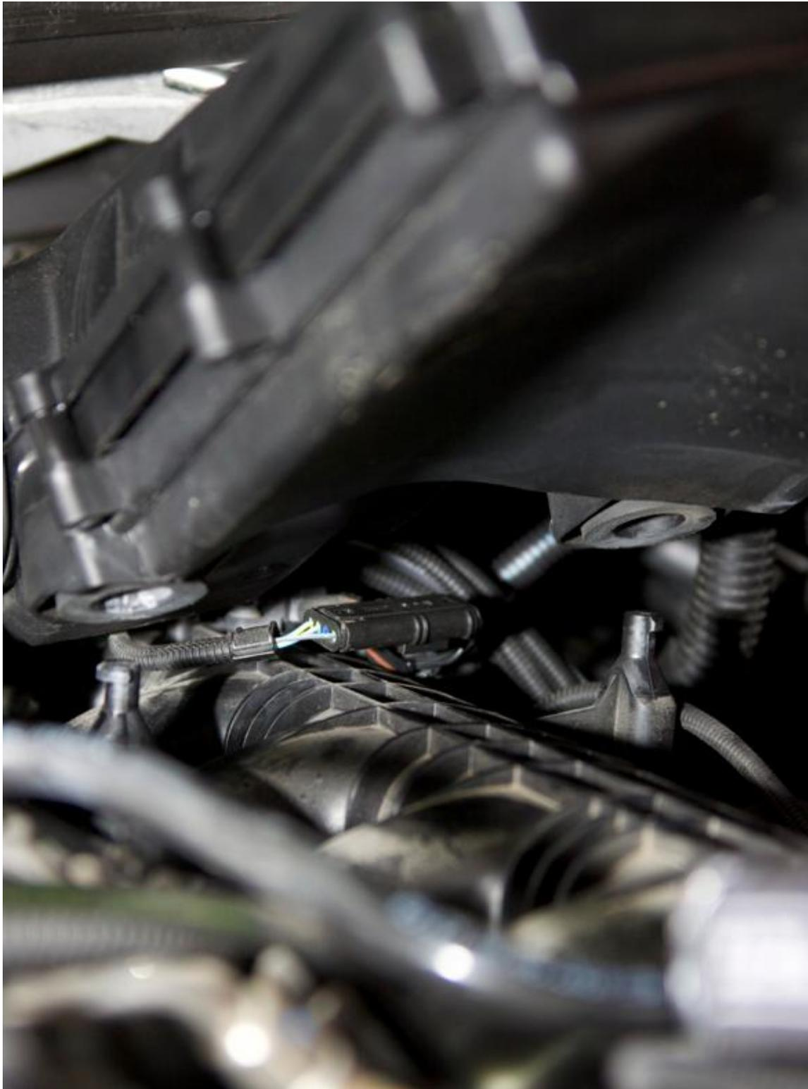
Sensor Two 2 - Use a very small screw driver to unclip the sensor, and install the piggy back sensors
