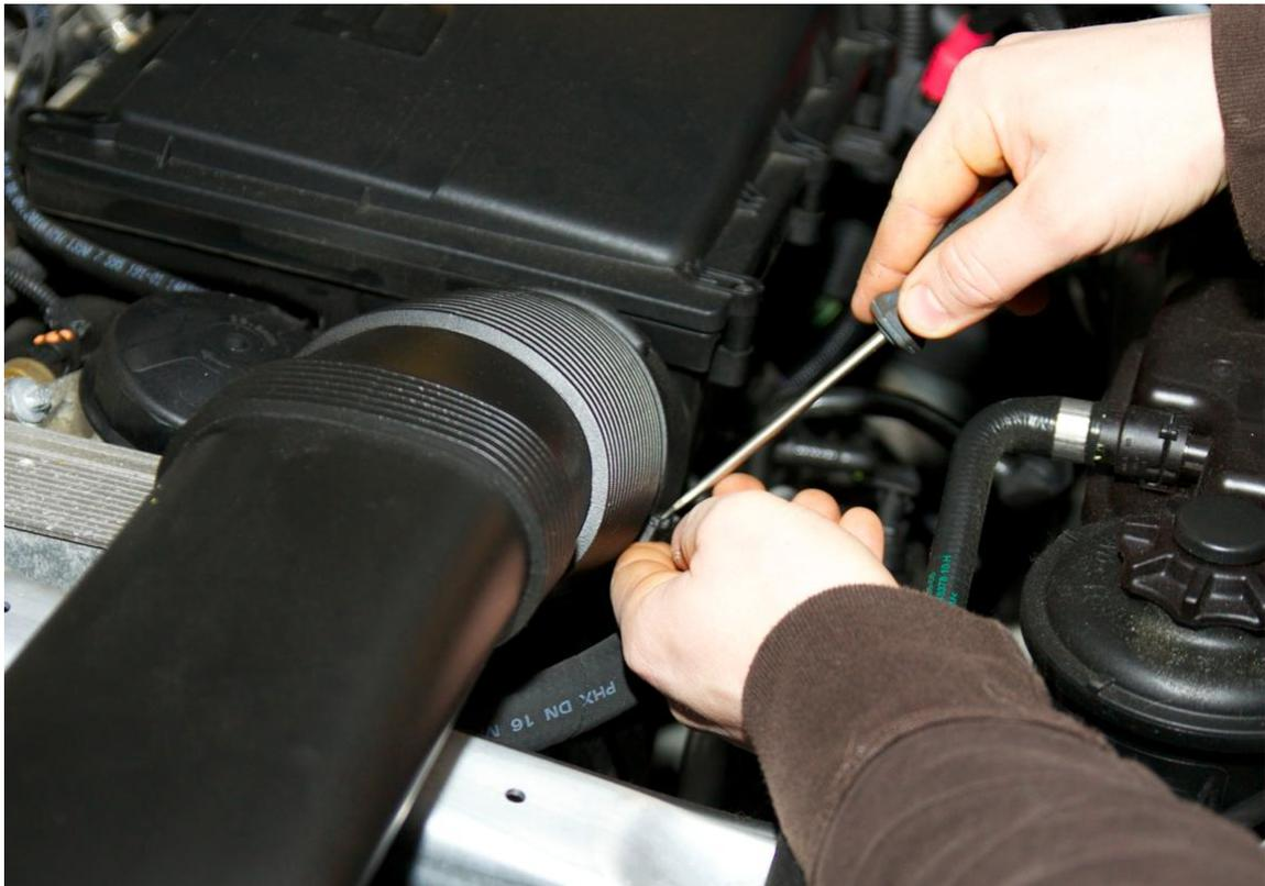
Air Box 3 - Unclip elbow
