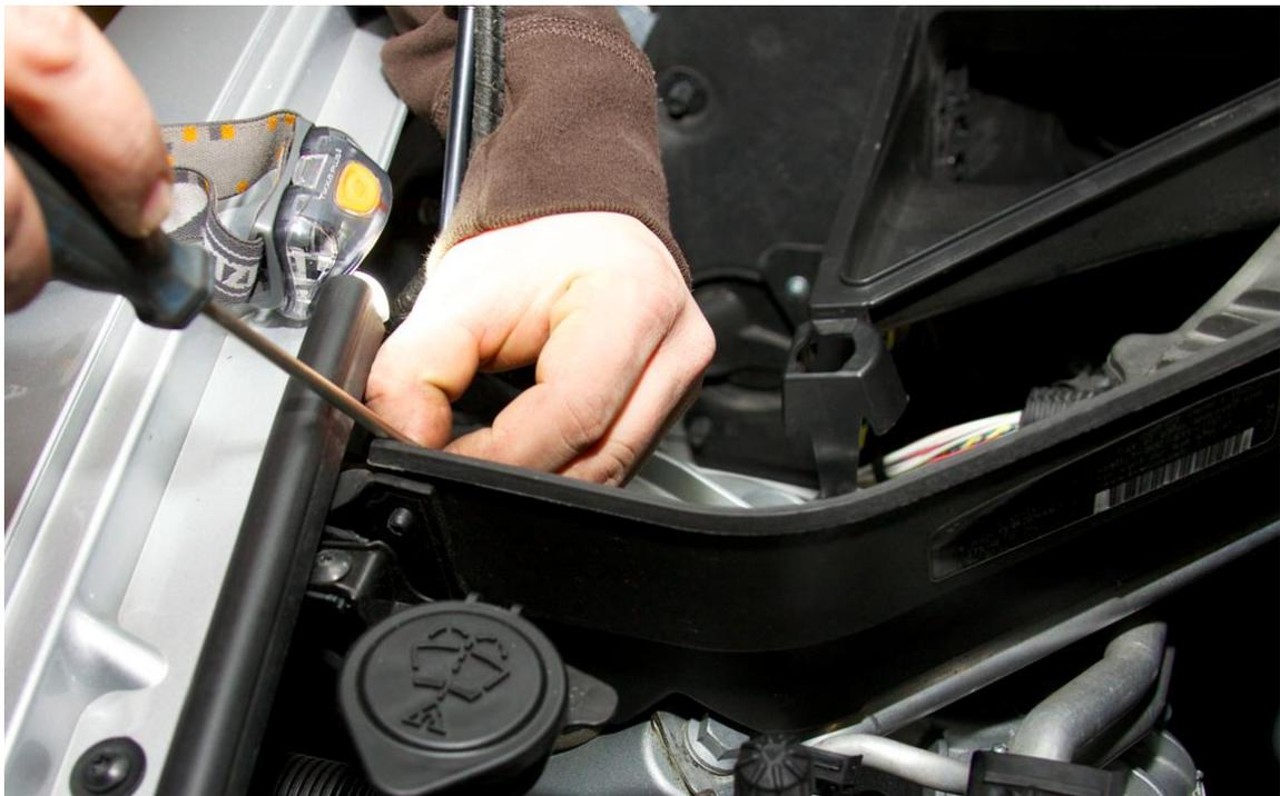
Control Module Install 7 - Take out the expansion rivet as well
