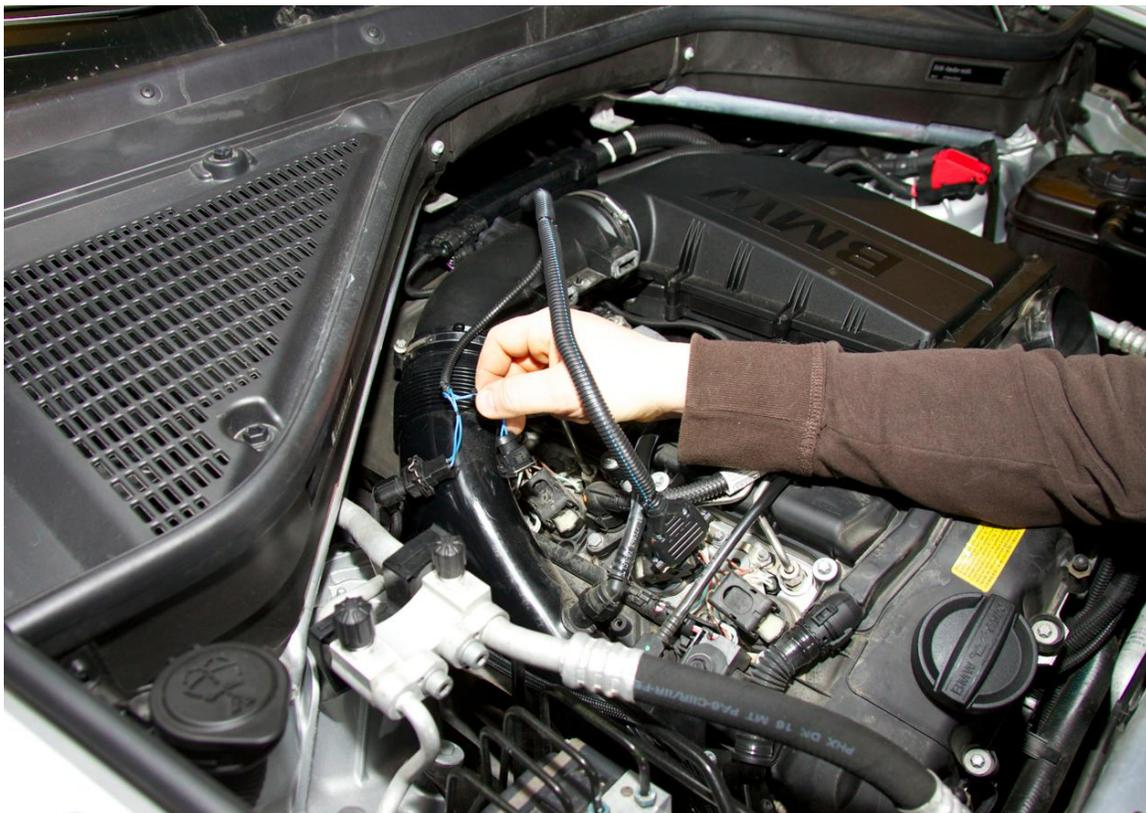
Sensor Four 2 Wire Routing Example
