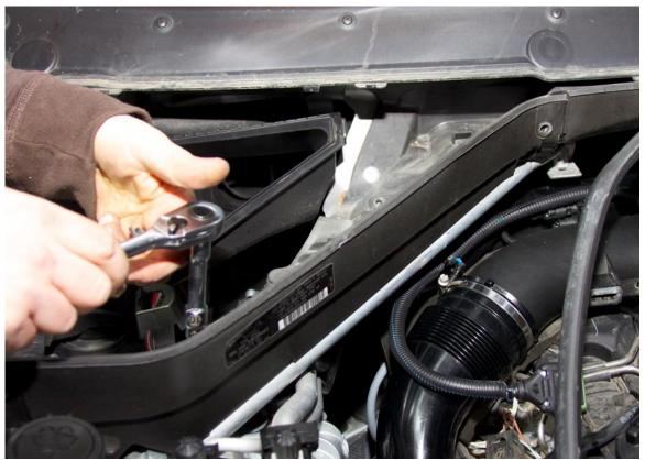
Control Module Install 6 - There is a combination of torx bits and two 10mm nuts
