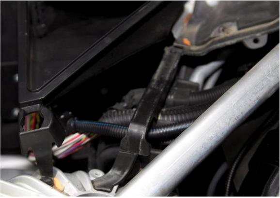
Control Module Install 13 - Fish through the harness and reinstall the black top piece
