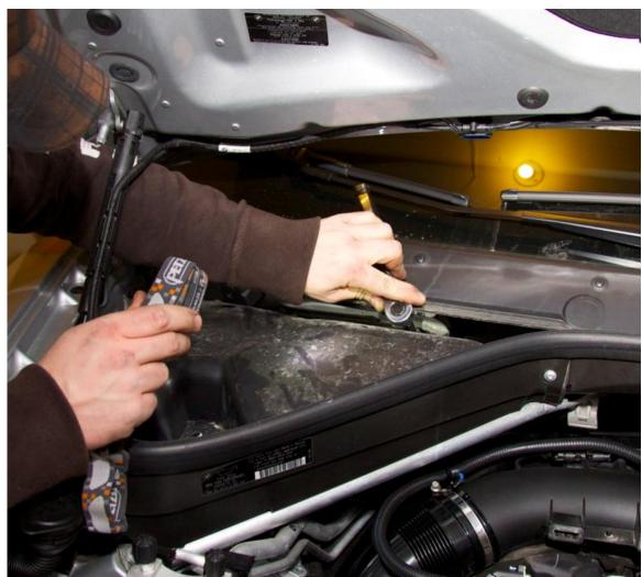
Control Module Install 3 - Uninstall the cabin air filter
