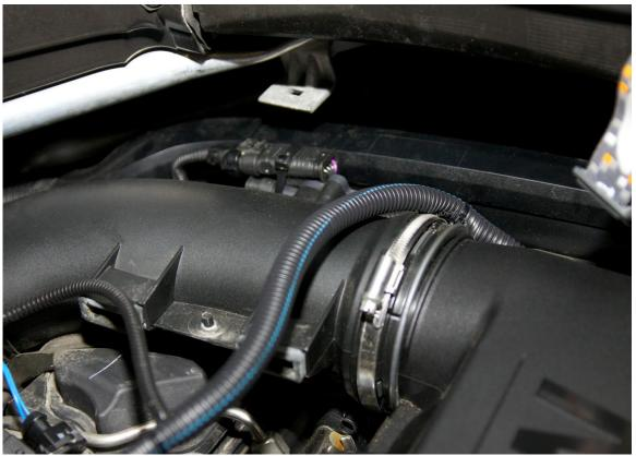
Sensor Three 3 - Take a small screw driver into the back of sensor three to loosen.
