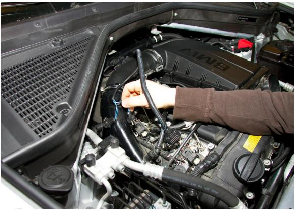
**Sensor Four 2 Wire Routing Example**
