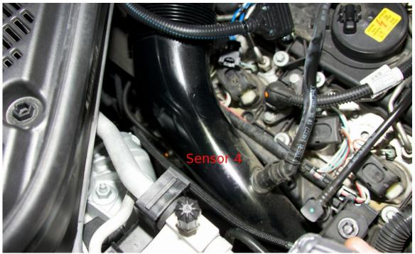
Sensor Four 1 - it can be spotted by the orange dot left of the black pipe. Thankfully, a spring clip secures this sensor. Just press on the spring clip to loosen this sensor.
