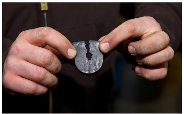
Control Module Install 12 - Cut open the rubber piece
