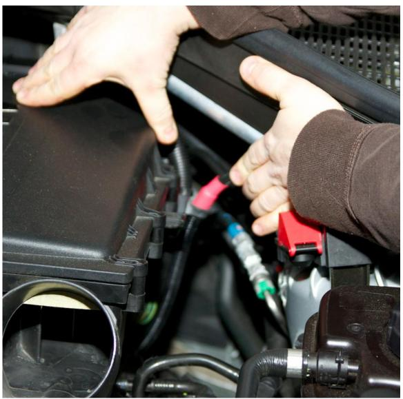
Air Box 4 - Unclip the wires from the side of the airbox
