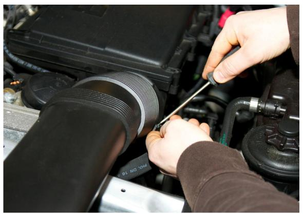
Air Box 3 - Unclip elbow
