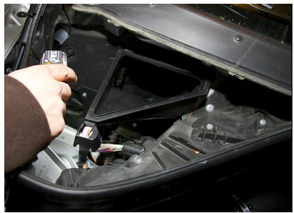
Control Module Install 5 - Take off the weather strip and the engine compartment divider
