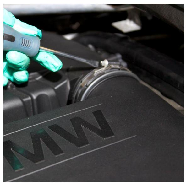
Air Box 1 - Loosen the clamp
