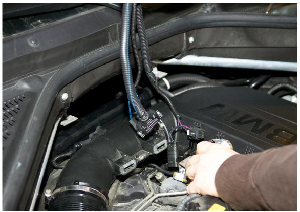
**Sensor Three 2 Harness Routing Example**
