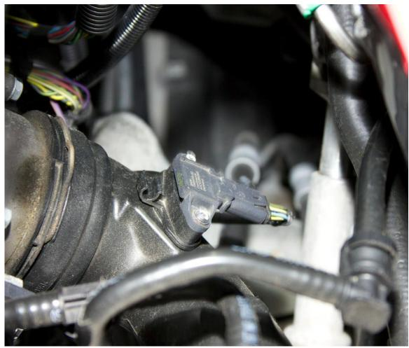
Sensor One 1 - Unclip the plug from the harness
