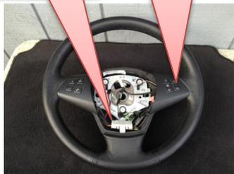
Complete heated steering with heat control module and controls
