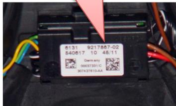
Heat control module. Steering with either white or black Module should work. PN 9217867-02 if you must know
