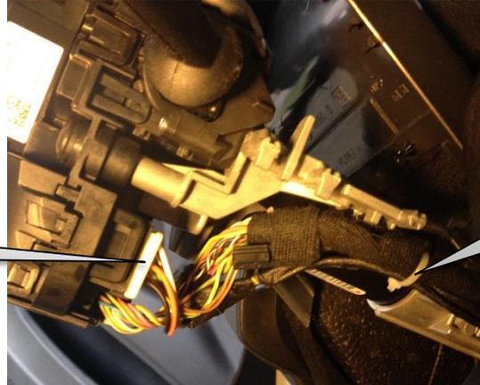
Plug 12 pin connector into coil spring
