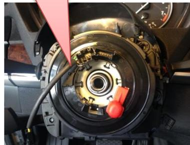
New coil spring cartridge With power harness
