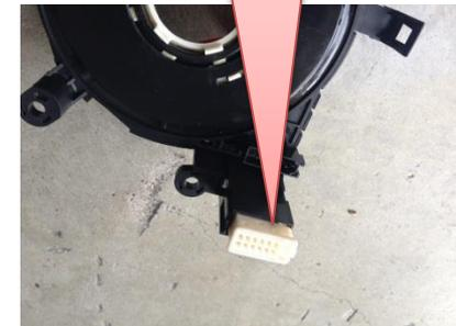
12 pin connector plugged into New coil spring. Old coil spring Has a 6 pin.
