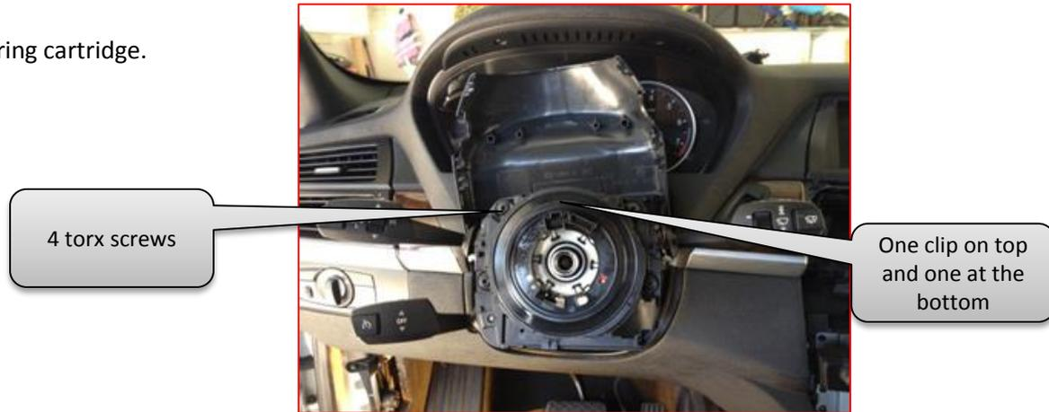
19. Install the new coil spring cartridge
