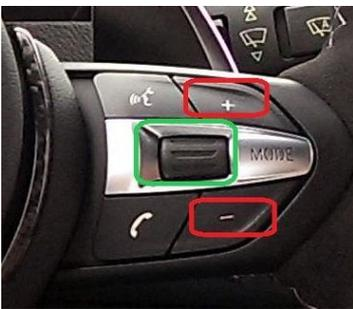
It can be done by pressing and holding **volume +** and **volume –** keys for 6-7 seconds. Backlight on the steering wheel will blink when mode is changed. Configuration will be retained after switching ignition off.
