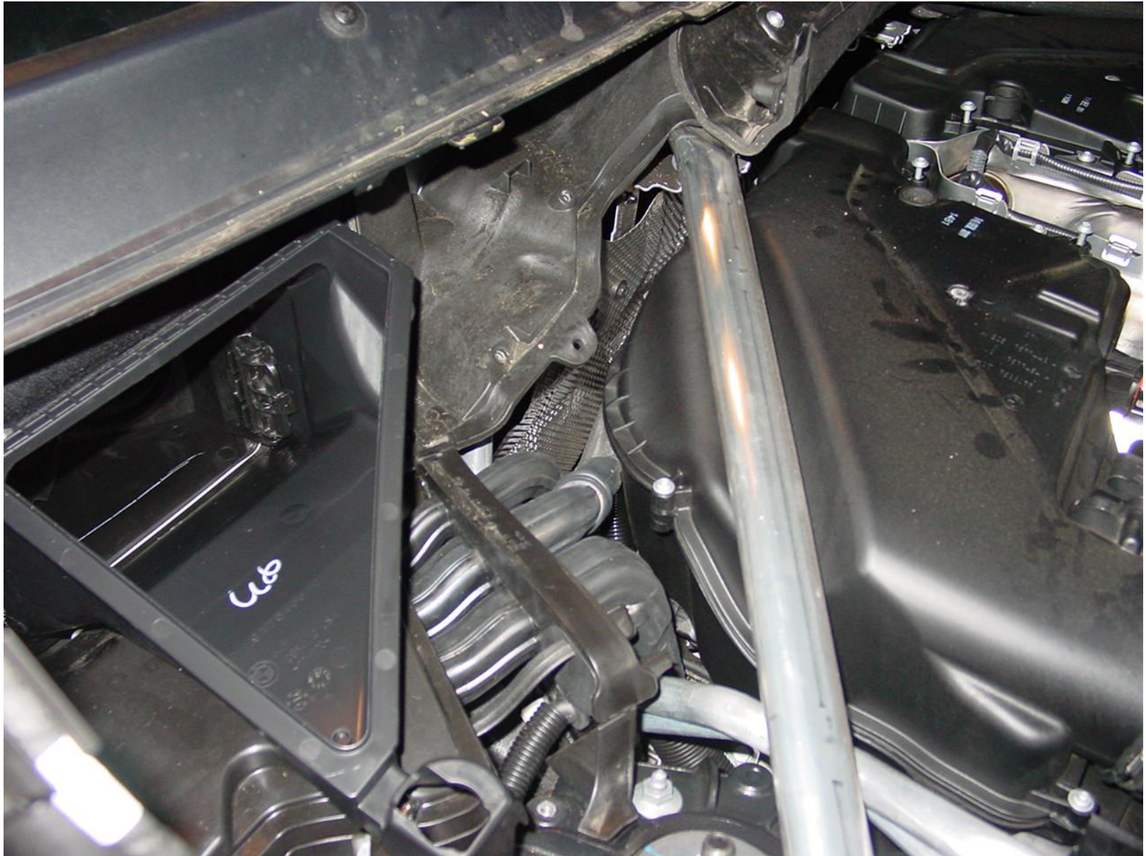
Left Side Divider Panel removed
