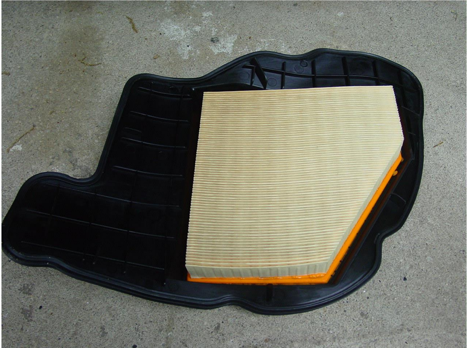
Right Side Air filter removed from air box
