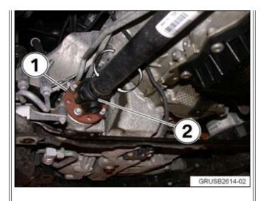
1. Checking the front U-joint:
