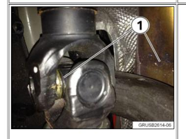
4. New Also check for excessive grease marks on the surfaces of surrounding components around the U-joints and for excessive grease released out of the bearing seals (1).
