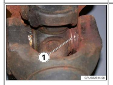
3. New There should be no excessive rust at the bearing seals (1). Note: There will be rust buildup on the driveshaft and mounting flange on some driveshafts. This rust is normal. Only excessive rust on the bearing seals indicates the seal may fail.
