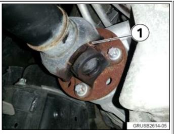
2. New There should be no exposed needle bearings (1).
