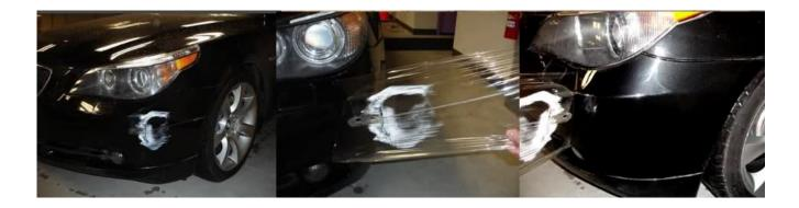
Even better... heres a quick 1 minute video showing a Gravelometer being using to test and demonstrate the films effectiveness (a device that hurls one pint of gravel (250-300 stones) at a painted surface at a velocity of 30-60 mph.
