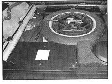
STEP 48 Secure the Battery Cover using the three #8 x 1" Sheet Metal Screws. Reinstall the floor panel.
