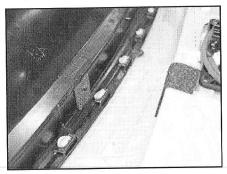
**STEP 10**Cut a second piece of the Foam Tape and apply it to the panel, over the clip as shown.
