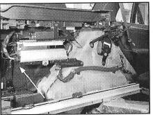
Pictured is the cargo area with the left side panel removed. Unplug the indicated factory amplifier plug for easier access to the factory wiring in **Steps 37-38**.
