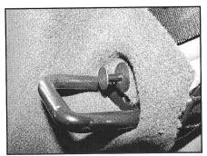
**S T E P 3 2**Remove the three clips that hold the side panel in place and remove the panel.
