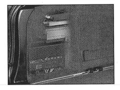
Cut the Foam Tape into three 4" strips, affix them to the new Battery Cover, and trim away the excess as shown.
