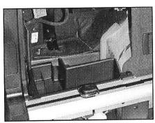
Remove the three clips that hold the storage pocket in place and remove the pocket.
