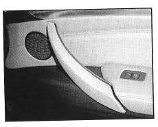
**STEP 4**Carefully pry off the trim on the pull handle and remove it from the vehicle.
