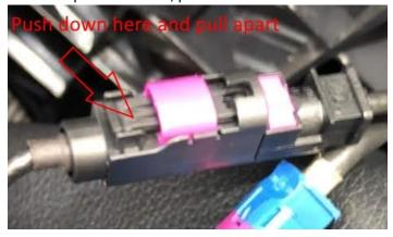
Large black connector, push down on black tab and then move lever until it 'clicks' Separate connection.
