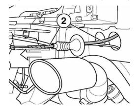
Re-seal grommet to hose/wires with electrical tape and re-connect hose to inline coupling.
