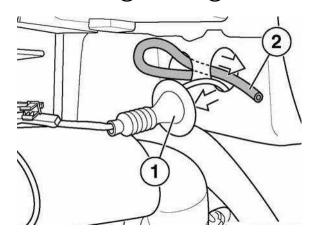
Using a fish wire, pull hose through other grommet alongside existing wiring.
