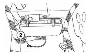
Connect the Helbako Trailer Control Module ① to the 16-pin plug of the hitch harness ②. If there is an available slot in the vehicle electrical panel, install the Trailer Control Module there. Otherwise secure it in the battery compartment.
