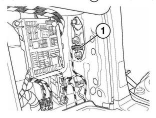
Locate the blue/brown wire 2 of the tail-light plug. This is the turn-signal wire.
