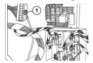
Locate the vehicle's 3-wire CANbus plug 2 shown below, and connect it to the 3-wire CANbus connector on the hitch harness. Note: the vehicle's CANbus plug may be taped flat against the rest of the vehicle wire bundle and it may be obscured by the fuse panel.
