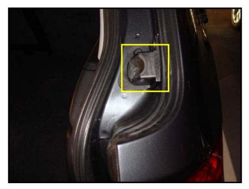
6. The bump stop adjustment is made from the outside area of the bump stop.
